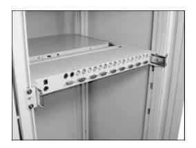
**9.** Slide the assembled drawer out. Push the KVM module box *evenly* toward the drawer, and then lock both units by the screws.
